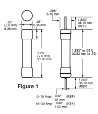
Figure 2 Dimension in mm.
